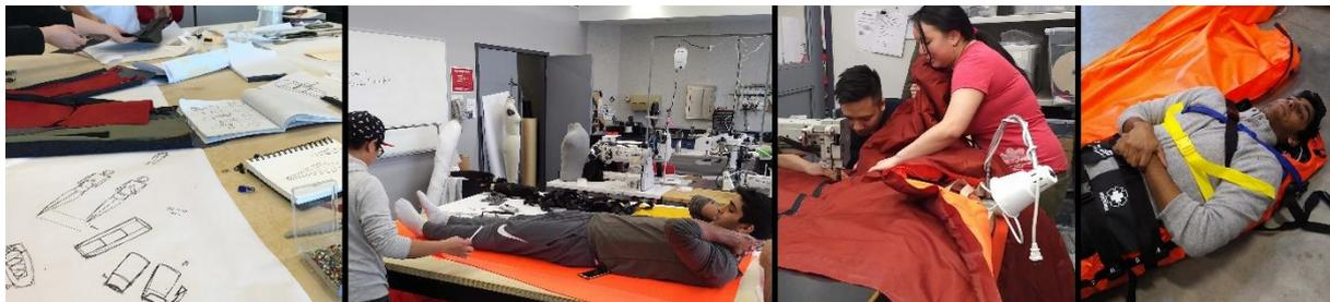
Figure 3. Iteration 1 - Small scale and full-scale prototyping of the Burrito: ideation development, anthropometrics, prototyping, and integration with medical equipment (image credits: Alisa Yao)
