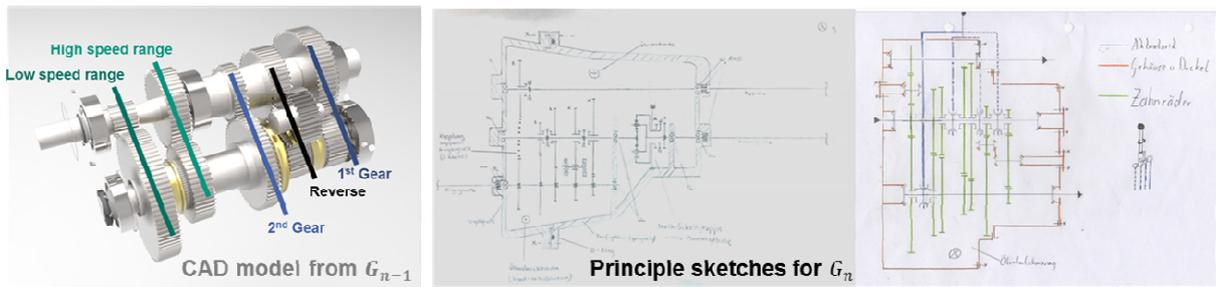
Figure 2. CAD model of the reference product ( $G_{n-1}$ ) for the subsystem “manual gearbox” and different principle sketches in the development of the next product generation ( $G_n$ )
