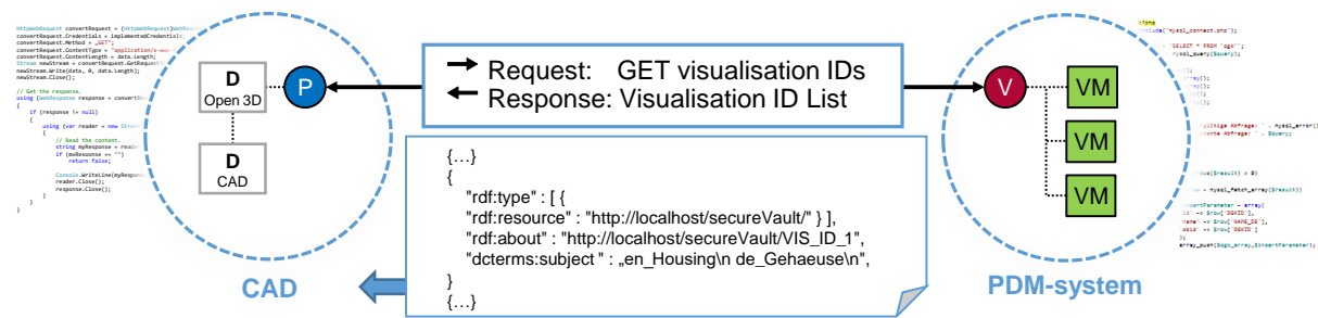
Figure 4: OSLC specification based request to get visualisation IDs from a data management system
