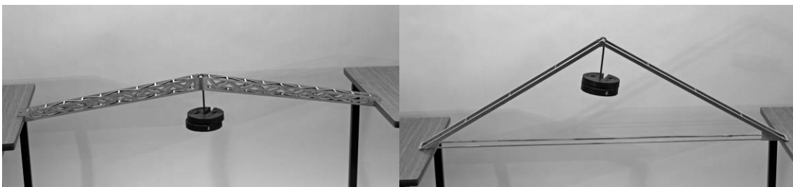
Figure 2. Compression structures using the tables or tension members to take side load
