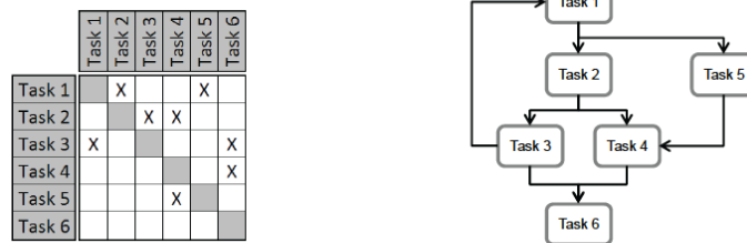
Figure 1: The Design Structure Matrix represents the dependencies in a complex system
