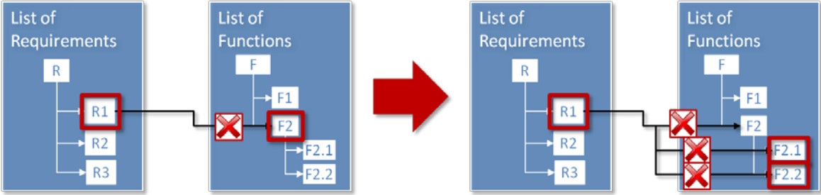
Figure 3: If there is no dependency between R1 and F2, no dependency exists between R1 and all child elements of F2.
