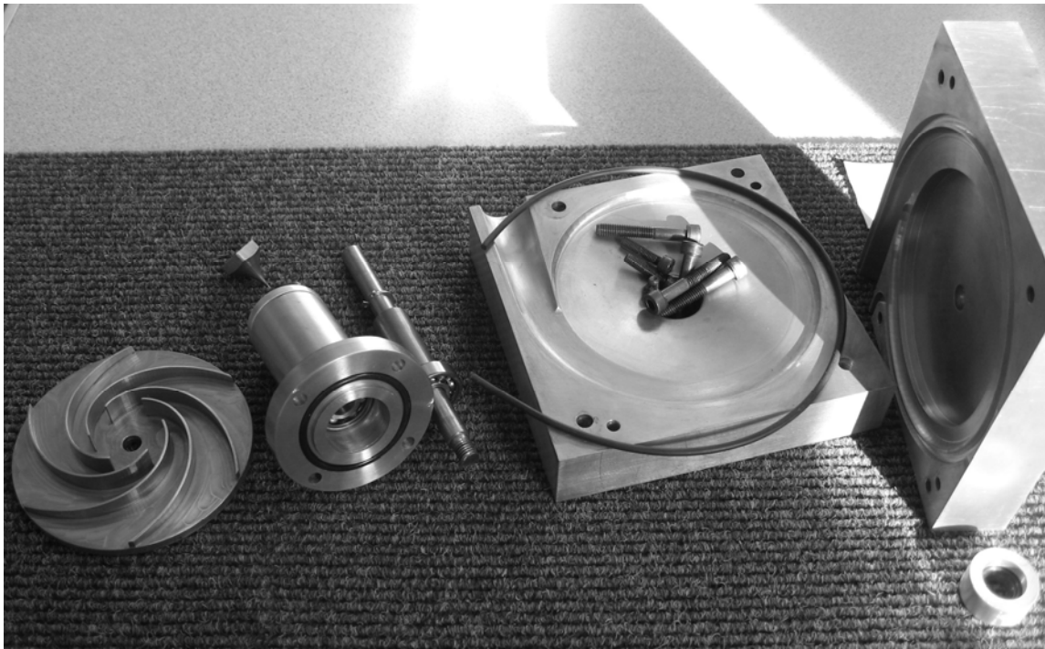
Figure 2. A typical set of pump components manufactured by the student group
