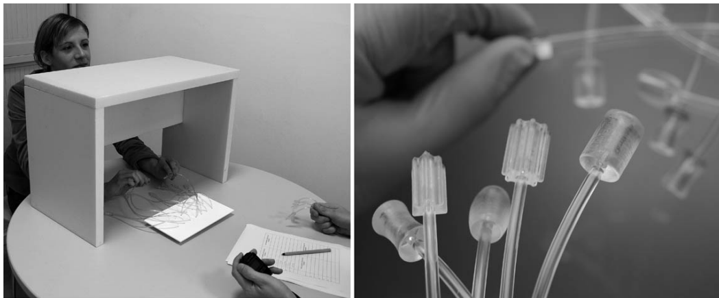
Figure 3. Haptic discrimination tests of connector shapes
