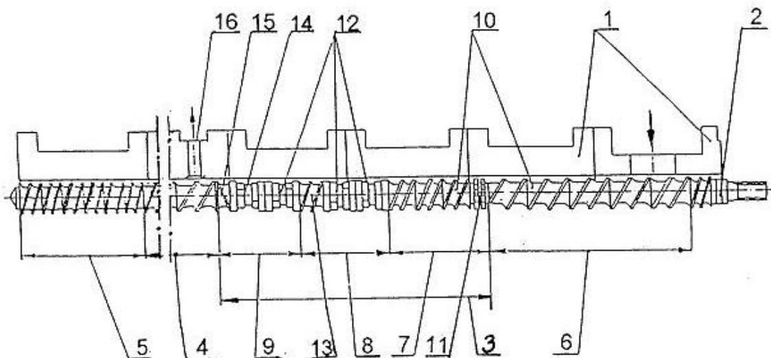
Figure 3. The outline of plasticizing system of the co-rotating twin-screw system: 1-cylinder, 2 – screw, 3 – plasticizing zone, 4– degassing zone, 5 – metering zone, 6– feeding zone, 7– preliminary compressing and heating up zone, 8– preliminary plasticizing zone, 9– intensive plasticizing zone, 10,13 – conveying screw elements, 11– mixing elements, 12 – kneading elements, 14– reverse conveying kneading elements, 15– reverse conveying screw elements, 16– degassing hole.
