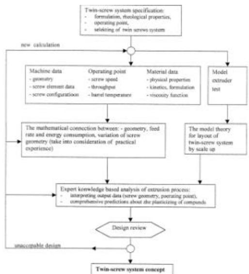
Figure 1. *Layout of the co-rotating plasticizing system.*
