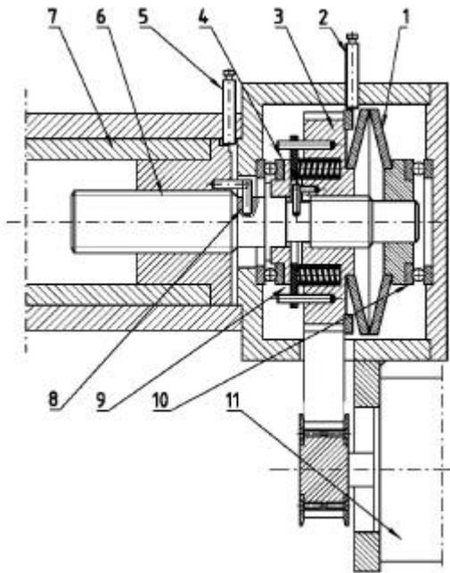
Figure 2. Screw mechanism for movements of a tailstock spindle.
