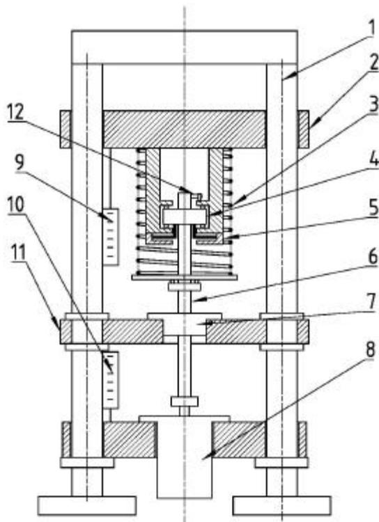
Figure 4. A press with a differential screw drive.
