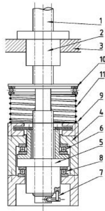
Figure 3. Differential screw drive.
