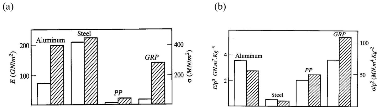
Figure 4. (a) Relative stiffness (open bars) and strengths (shaded bars) in flexure of equal thickness sheets from the materials. (b) Relative stiffness (open bars) and relative strengths (shaded bars) in flexure for sheets of equal weights from the materials. [7]
