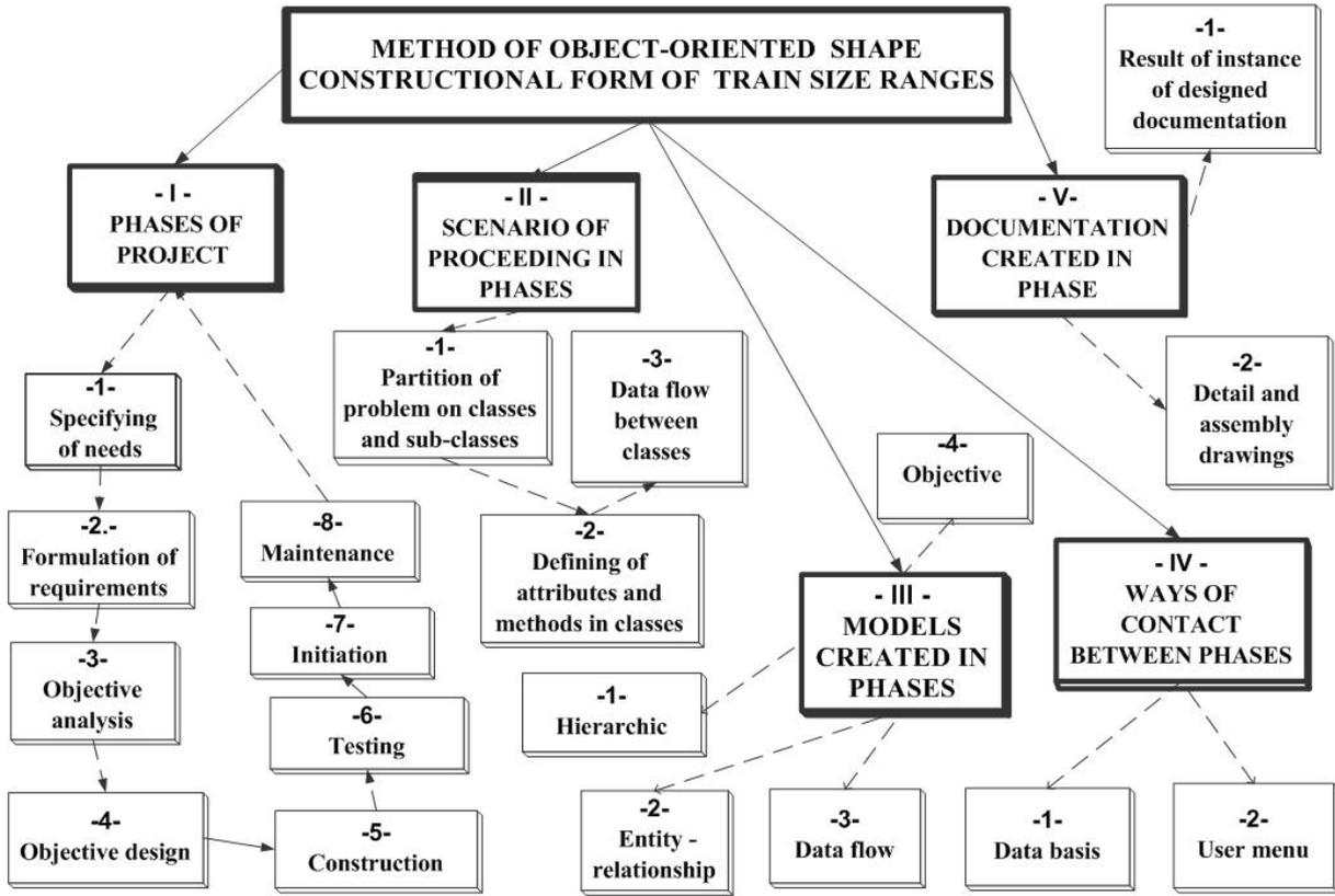
Fig. 3. Elements of design process and output of offered method
