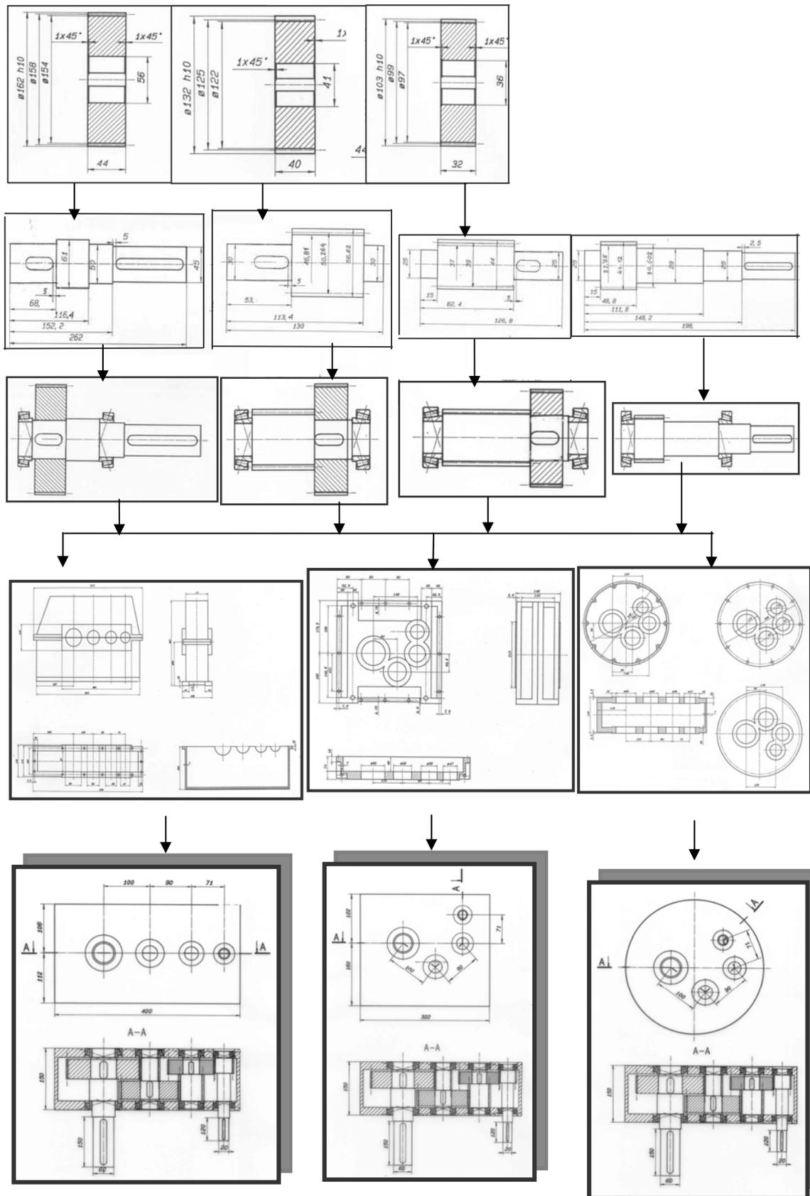
Fig. 5. Scheme of objects of three-stage spur train according principle "from an overall view to the details"
