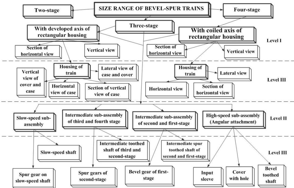
Fig. 4. Scheme of hierarchical model of size ranges of three-stage bevel-spur trains
